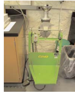
Dr. Taylor's lab houses Hege Seed Treater, which kept more for historical purposes. It isn't used much today because the Rotary Pan and Film Coating machines are far more accurate.
