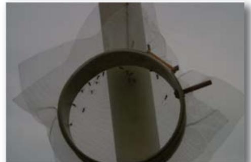
Mosquito bioassay cage to field test adulticide efficacy. Courtesy AFPMB.
