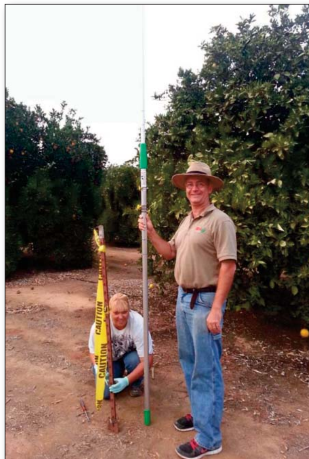
Western Region Researcher, Keri Skiles & IR-4 Public Health Pesticide Manager, Karl Malamud-Roam, set up a droplet sampler for measuring incidental deposition on crops from mosquito control sprays.
