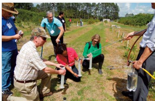
IR-4 study director Ken Samoil, SOR field coordinator Michelle Samuel-Foo, and Field Research Director at TX Agril Life Weslaco, Cristina Marconi, capture the output from a boom during a calibration event as part of the field demonstration at the University of Florida horticulture science facility. Photo by Jun Estorinos
