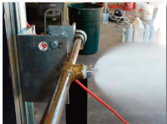
GLP testing of spray equipment for novel data collection efforts to support mosquitocide registration.
