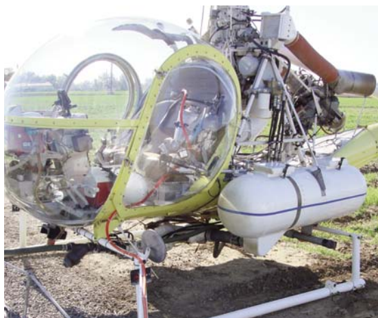
Parked Helicopter outfitted with rotary atomizer (Becomist) nozzle from CO 2 tank on seat. Photo by Stephen Flanagan.
