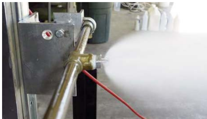
Calibrating 20 micron droplets with laser and wind tunnel for mosquitoicide residual study. Photo by Clint Hoffman
