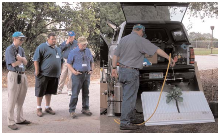
Participants look on as Wayne Curry of Weed Systems Equipment (r), uses an artificial plant, to demonstrate the spray distribution pattern of various nozzles.
