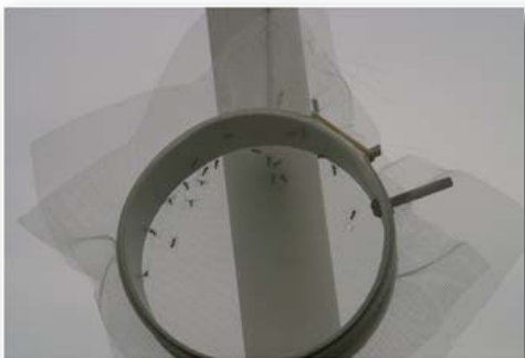
Mosquito bioassay cage to field test adulticide efficacy. Courtesy AFPMB.
